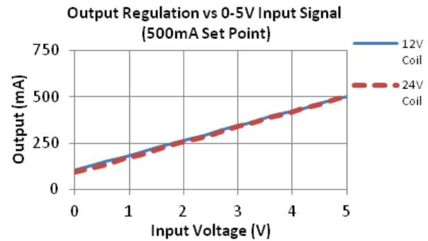
Note: All the above readings were taken with the DEC005000 adjusted for a .5 Amp maximum output at 100 Hz. A 14.6V supply was used for 12V coil tests and a 26V supply was used for 24V coil tests.
